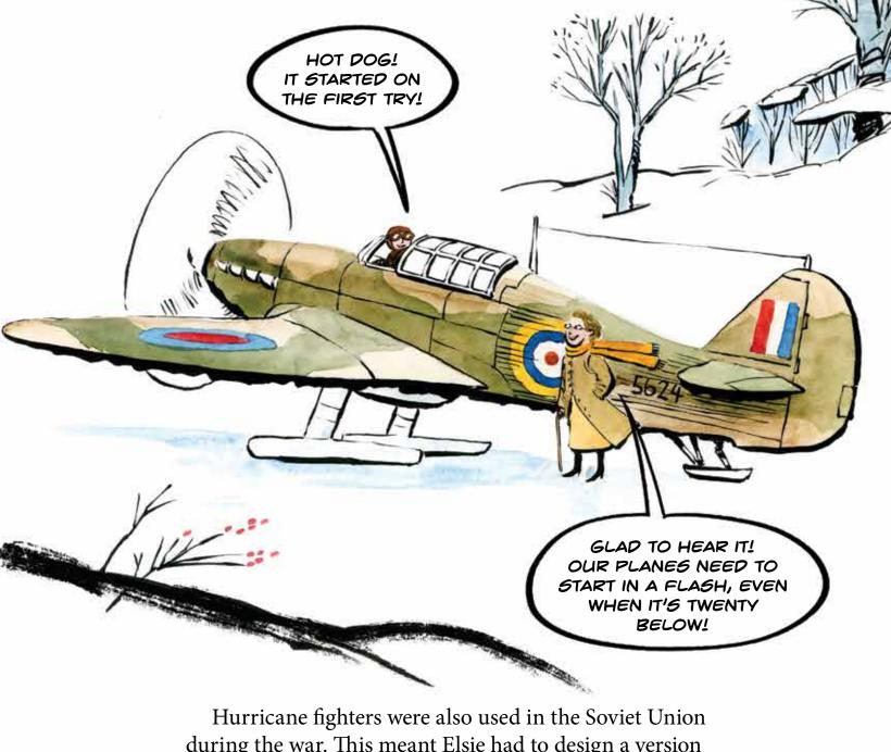
Hurricane fighters were also used in the Soviet Union during the war. This meant Elsie had to design a version of the plane that could fly in icy weather. She added skis so the plane could land on snow, and fitted de-icing systems on the propellers, tail and wings. Back in the 1940s, it was very unusual for a woman to be in charge of such a technical project. Elsie became famous around the world.
